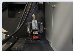
Printing material automatic height detection device
