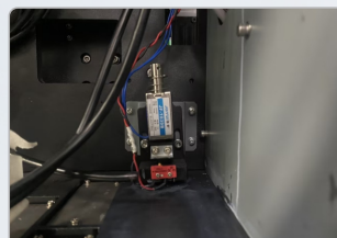
Printing material automatic height detection device
