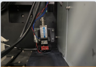
Printing material automatic height detection device
